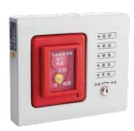
The GS8204 addressable manual/ auto switch is an important part of a gas release system as well. Under the manual mode, the gas will not be released even if the alarm has been triggered. Under the auto mode, the gas releasing will be based on the settings and programming. It will be set to manual mode when someone enters the protection area. GS8204 is an addressable device, direct connect to gas release control panel 2<sup>nd</sup> communication bus.
